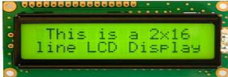
Gambar 2.14 LCD (*Liquid Crystal Display*) 2x16
