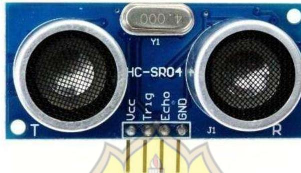
Gambar 2.3 Sensor *Ultrasonik* HC-SR04
