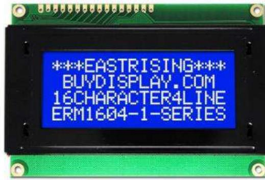
Gambar 2.6 LCD 16X4
